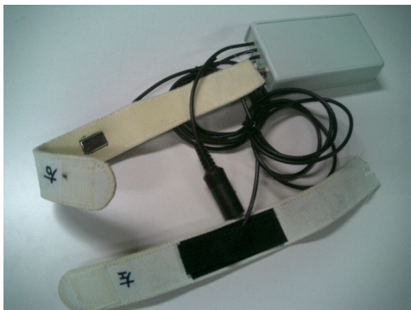
Figure 6: Dual 3-D acceleration sensor
