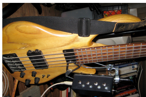
Figure 4: The control box mounted to an electric bass.
