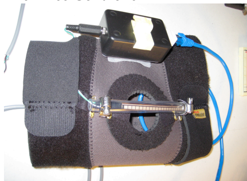
Figure 2: The knee controller uses a bend sensor and accelerometer.
