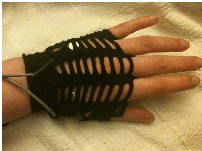
Figure 1: Simple glove with vibration motors, which connects to a laptop via an Arduino.
