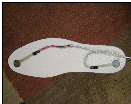
Figure 3: Foot controller using two FSR's.
