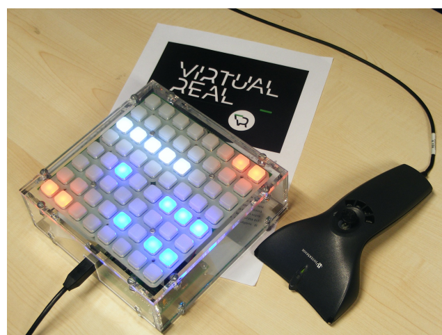
Figure 6: A 3D wand and a 40h Monome assembled from a kit were plugged into the system as off-stage audio/visual controllers.
