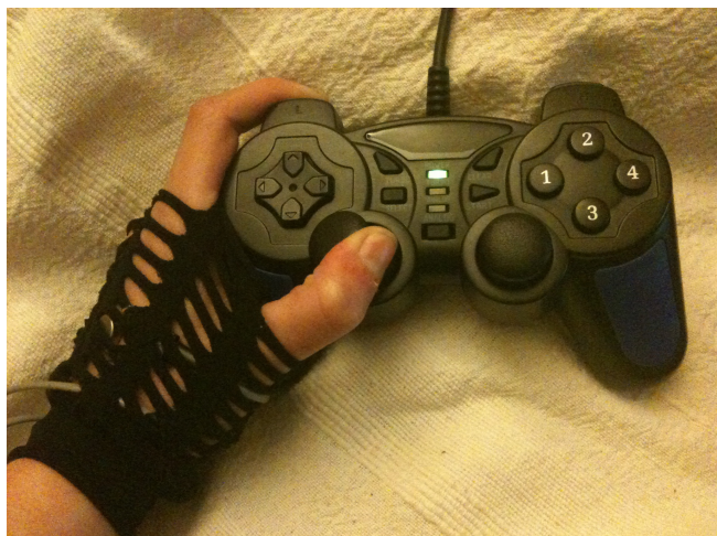
Figure 2: Vibrotactile feedback used in conjunction with generic game controller.
