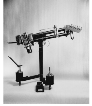
Figure 3: Aglaopheme , a slide guitar robot
