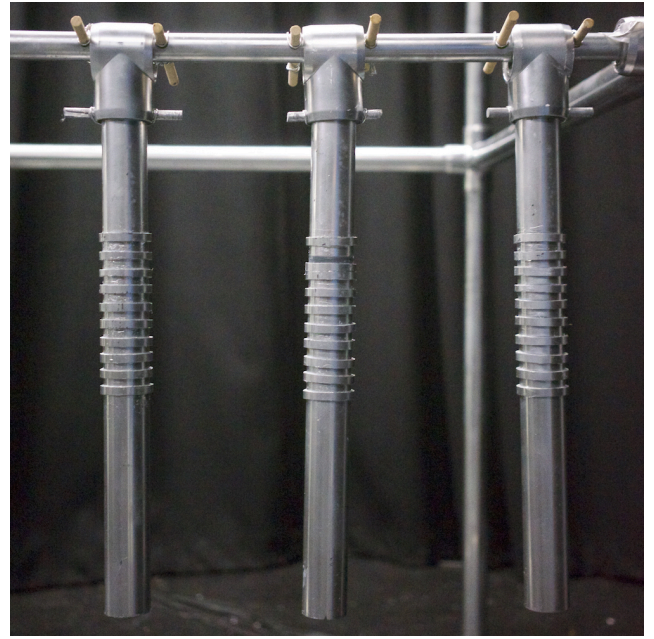
Figure 3: Close-up of pendulums, 50 centimetres long, with ten raised rings at one centimetre spacing.
