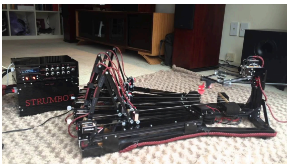
Figure 6: StrumBot, a multi-string chordophone
