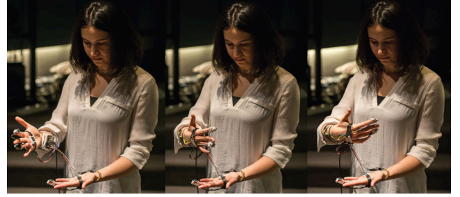
Figure 5: ASL music gesture creates beating effects with waving the hand captured through accelerometer worn on the right hand.
