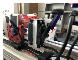
Figure 8: MechBass' servomotor-based damper
