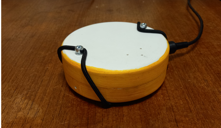
Figure 4. The tambourine makes sounds when it is tilted in any direction.
