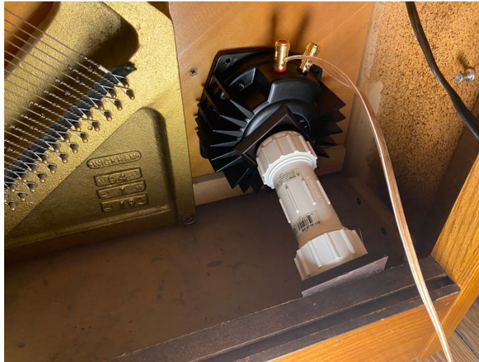
Figure 3. The shaker is attached to the soundboard through the use of a tension rod.
