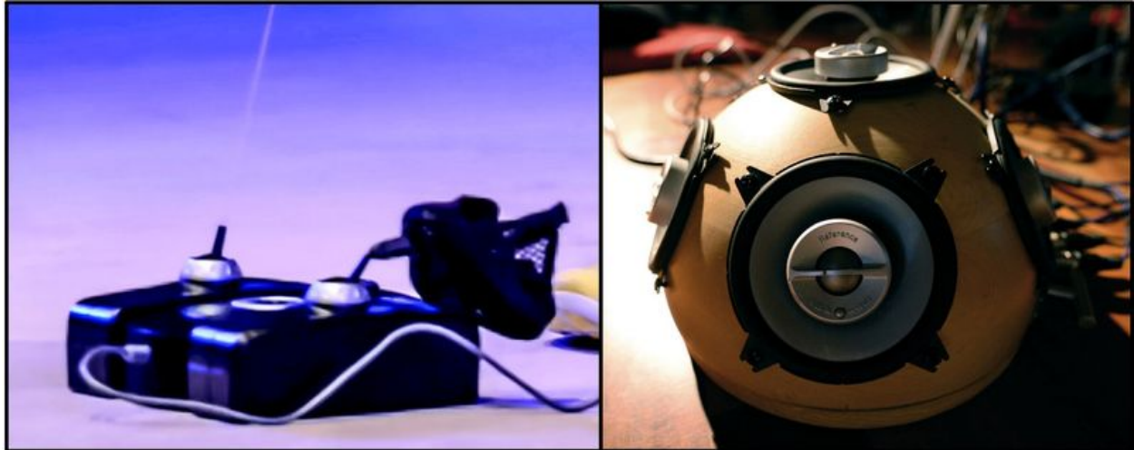
Figure 2. (a) GameTrak Tether Controller and (b) Hemispherical Speaker with Subwoofer.
