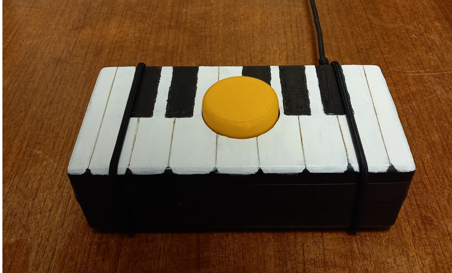
Figure 2. The piano, featuring a single yellow button for interaction.
