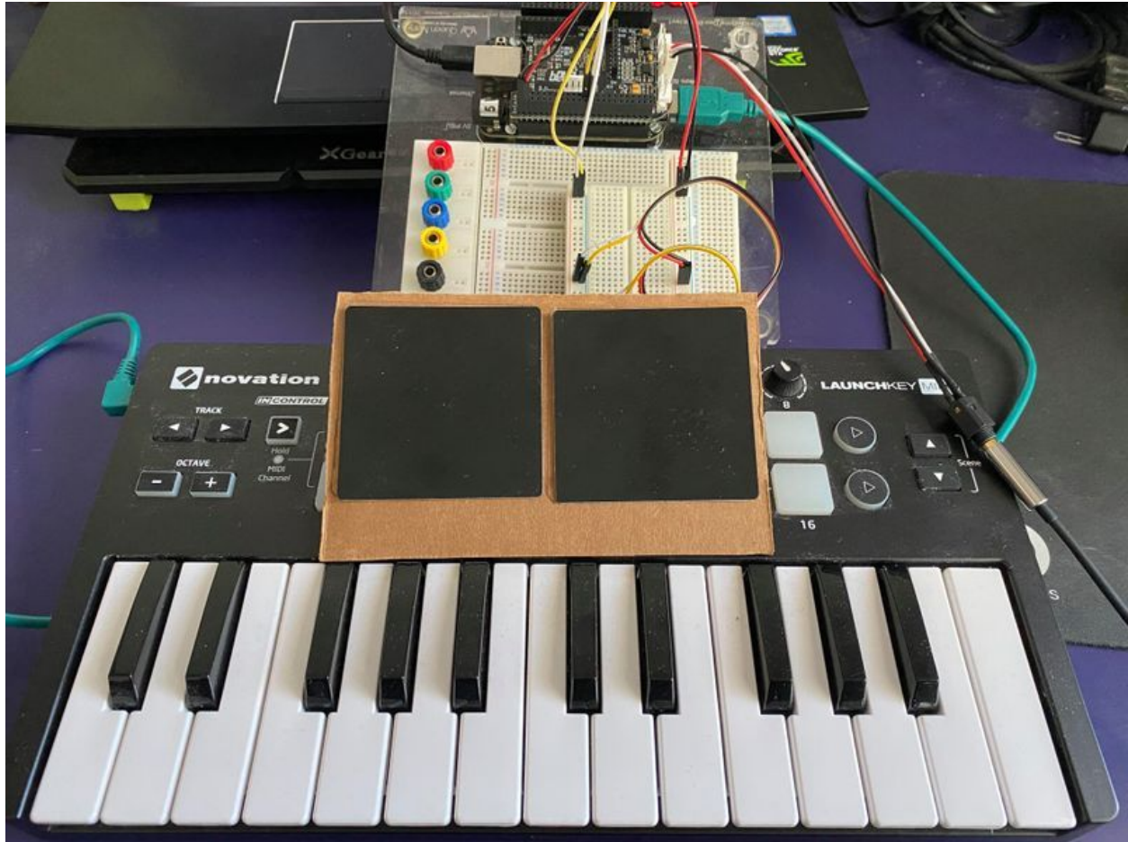
Figure 1: Original prototype of the Timbre Explorer, featuring from top to bottom the Bela microcontroller, two 2-dimensional touch surfaces and a MIDI keyboard.
