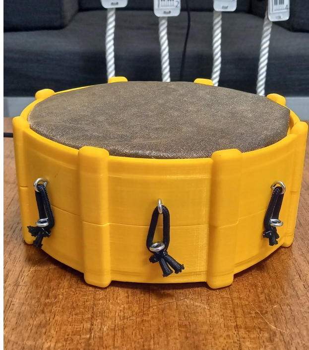
Figure 3. The drum is played by touching the conductive membrane on top.
