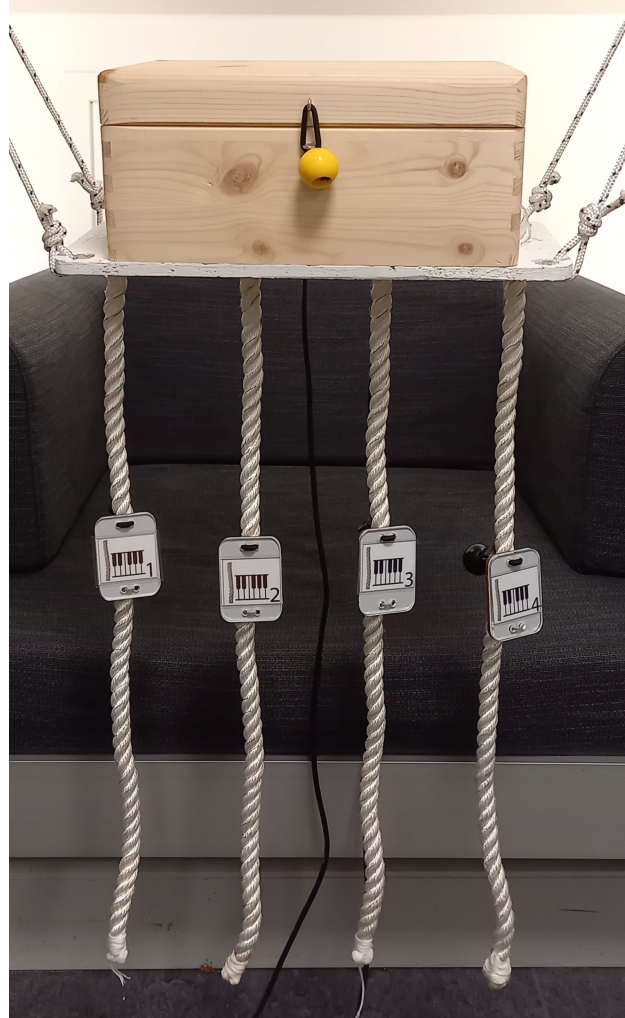
Figure 5. The rope synthesizer is played by touching or holding the ropes.
