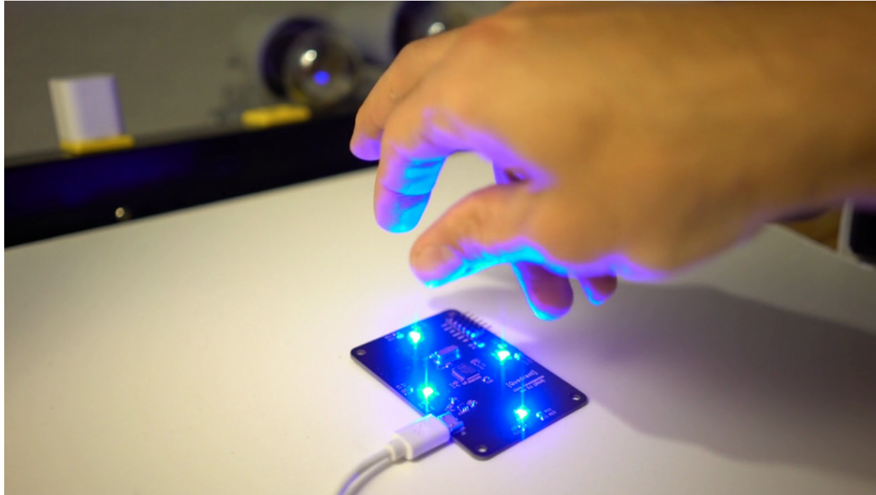
Quadrant PCB, showing micro-USB connector, STM32 microcontroller (center), distance sensors and feedback LEDs (blue diamond pattern).
