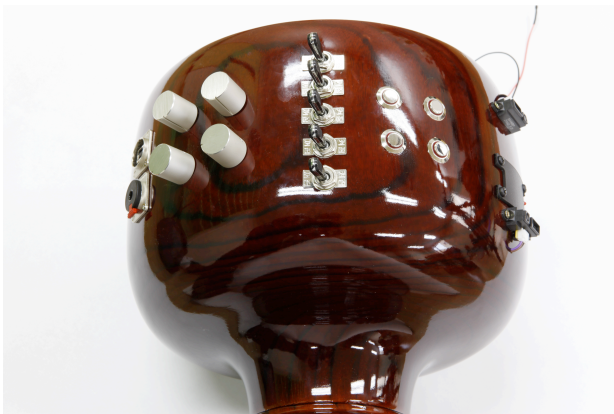
Figure 6 - eJanggu showing placements of embedded USB jack, knobs, switches, buttons, IR sensors
