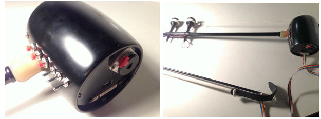
Figure 3 - eHaegum final design with electronics installed inside the traditional instrument.
